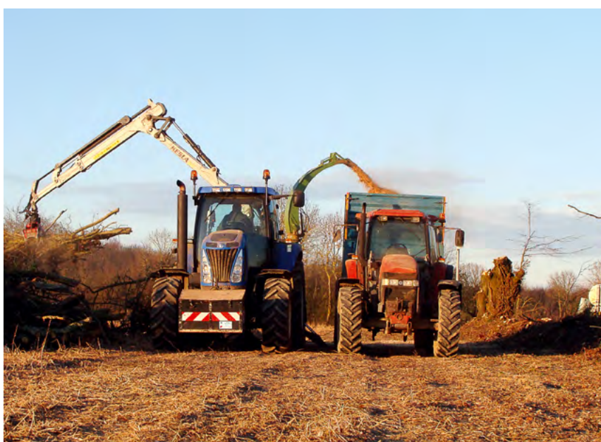
Ramial chipped wood is produced by crushing pollards branches Ref: D. Mansion
