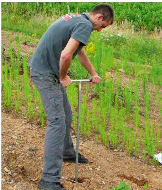
Using an auger to collect soil cores as part of an agroforestry assessment (Ph. Gaudry – CNPF)
