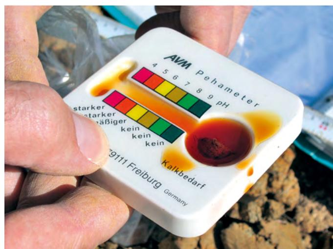
On the field the soil acidity is measured with a colorimetric pH-meter. If the soil is too acidic, it will be more difficult for the trees to capture the minerals. A high pH value usually indicates the presence of active limestone content
