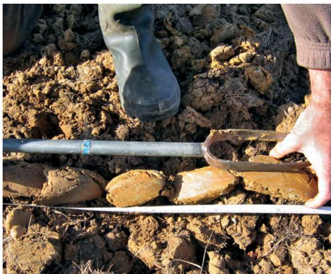
Soil core samples are collected by auger from the surface down. The whole soil is reconstituted by juxtaposing the successive soil core samples
