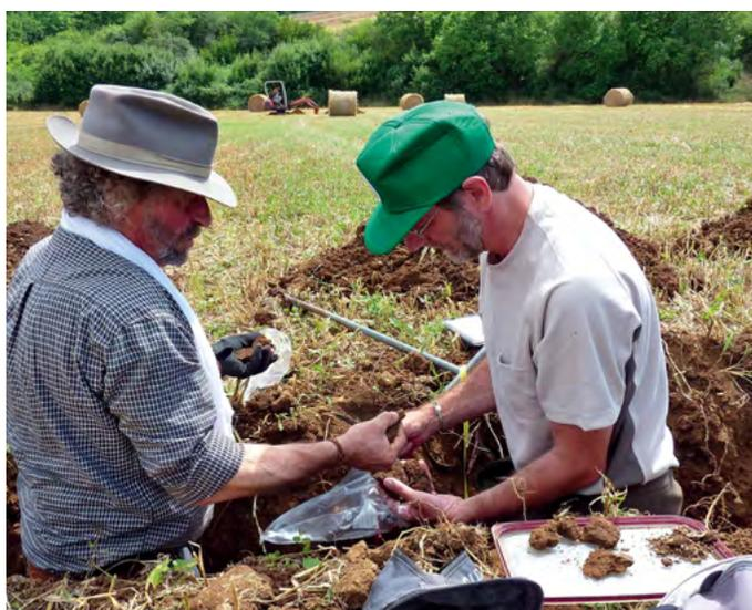
The soil pit enables a carefully observation of soil horizons and makes possible soil sampling for laboratory analysis, both chemical and physical
