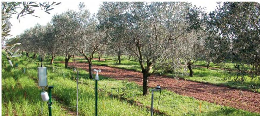
Continuous microclimate measurements (air and soil temperatures, relative air and soil humidity, wind speed, and incident photosynthetic active radiation) are carried out in the agroforestry trial (INRA Mauguio, France.) Ref: D.Desclaux
