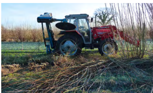
Willow coppice harvested with circular saw
